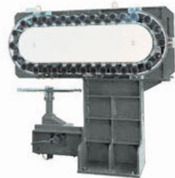
24 tool ATC rotary tool magazine
