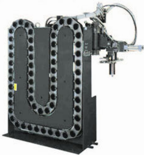
Horizontal and vertical ATC hydraulic tool magazine
