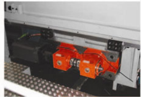
DCMS series machines are precision gear driven when X axis travel is longer than 11M or displacement is faster than 10M/min.
