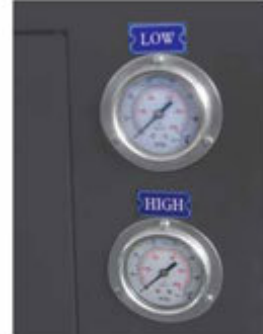
High and low pressure of hydraulic chuck
