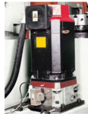
High torque main spindle motor with built-in dual speed gearbox
