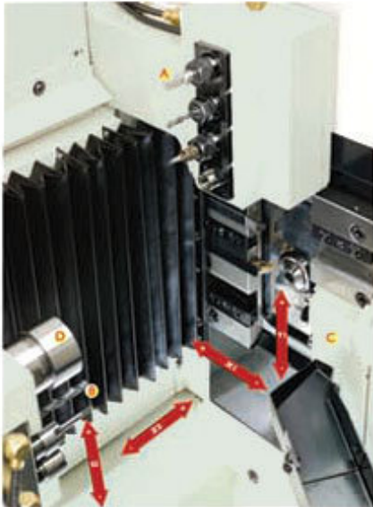
A: Back Driven Tools (4pcs) B: Face Driven Tool (1pc) C: Cross Driven Tools (3pcs) D: Subspindle
