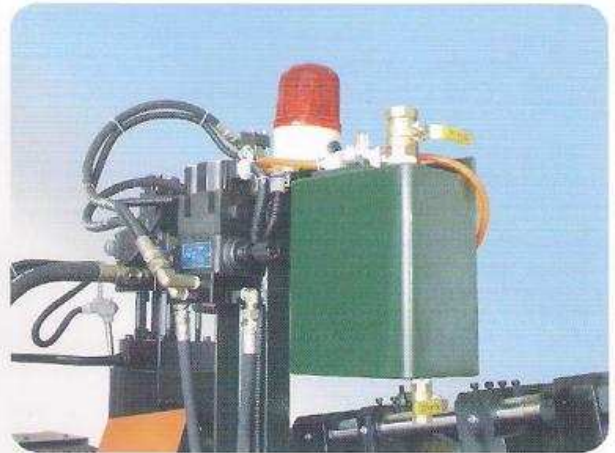
大容量離型劑罐：避免以前小容量頻繁添加脫模劑的繁瑣 Large capacity mold release tank: Avoid frequent mold release agent adding trouble with small capacity tank,
