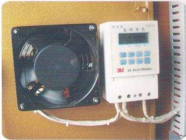
微電腦自動熔料：可在停機後隨意設定以後的熔料時間 Microcomputer automatic melting: Can set the material melting time freely after machine stopped working.
