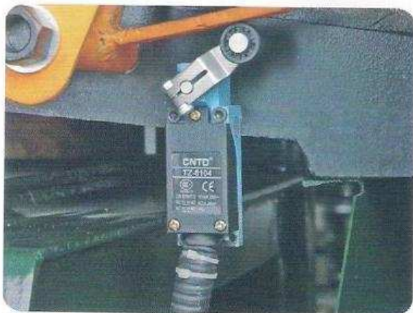
安全門開關：避免因疏忽或生產操作出現故障 Safety cover switch: Avoid operation faults caused by carelessness.
