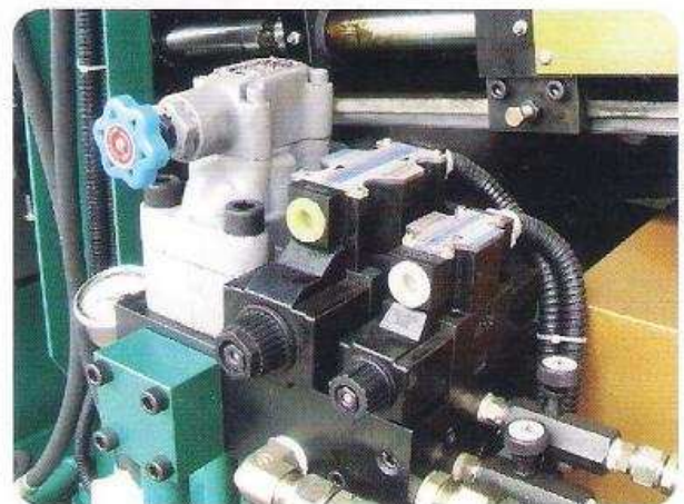
特設卸壓裝置，可有效保護油泵及電機，延長其使用壽命。 Special pressure relief device, can protect oil cylinder and electric motor effectively and extend service life.
