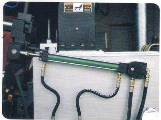
進退座油缸式：解決進退座的煩累，更加方便快捷 Seat in and Seat out cylinder: Easy and fast on cylinder forward and backward.
