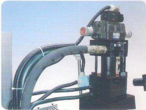
壓射軟管式：避免傳統無縫管焊接式因壓射產生的漏油現象、確保壓射的平穩 Injection hose: Avoid oil leaking accidents caused by injection from welded seamless tube design of traditional machine.
