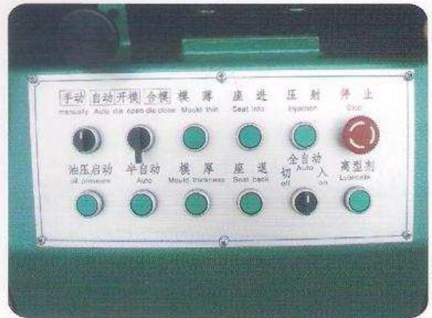
開模合模開關採用三段自動復位式避免傳統二段式造成的開合模線圈經常燒壞的弊病，採用德國西門子產品 Mould open and Mould close switch adopts 3-level automatic reset switch design, avoid mould open & close coils burnout problem with traditional 2-level switch, adopts Siemens products imported from Germany.
