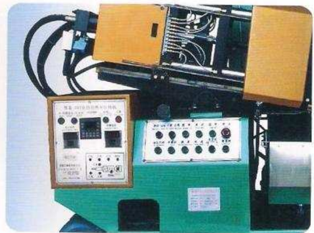
全電腦一體化控制,可編程及遠程控制,無須以太網卡; 採用美國H3ORNEA\OCS控制器,中英文顯示;實時控制, 輕鬆采集生產數據 Computer integrated control, programmable and remote control, no Ethernet card; Using the United States H3ORNEA \ OCS controller, displaying Chinese or English; Real-time control, easy to collect production data
