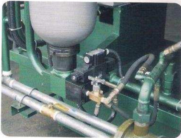
氮氣瓶座連體型：避免傳統機器管接式因壓射震動產生的震裂漏油現象 Combined Nitrogen gas cylinder seat: Avoid oil leaking accidents of shatter crack caused by injection vibration from pipe coupling design of the traditional machine.
