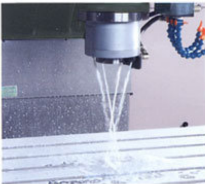
Coolants Jets Around Spindle
