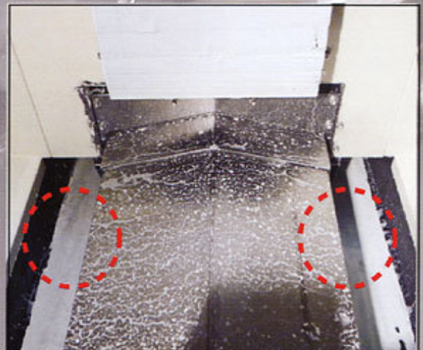
SPECIAL DESIGNED CHIP OUTLET FOR CHIP REMOVAL.
